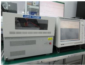
Fig 4. Actual image of the ammeter and the voltage source represented by an in-house curve tracer.
