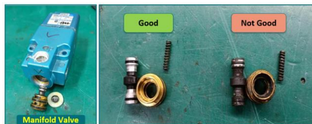
Fig. 17: Defective Manifold Valve
