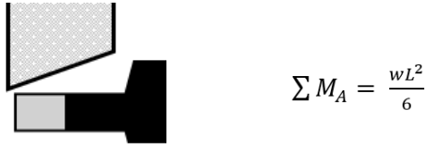
Figure 19. (Left) A new triangular dambar punch to which the total load (Right) it can be computed using the new bending moment formula.
