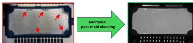
Figure 1: Post-mold cleaning effect on substrate with mold flash
