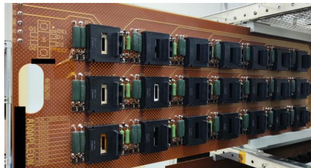
Fig 3.3 Sample burn-in load board
