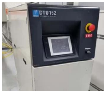
Figure 9. Water Temperature Control Unit (DTU) 4 . Sawing machine accessory which help to control the Cutting water Temperature.
