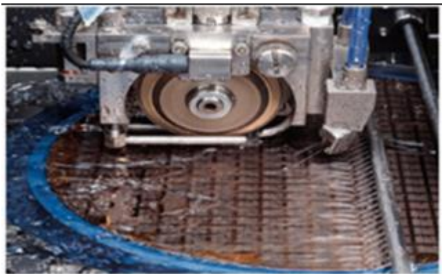
Figure 2. Demonstration of Mechanical Wafer Dicing Saw Process.
