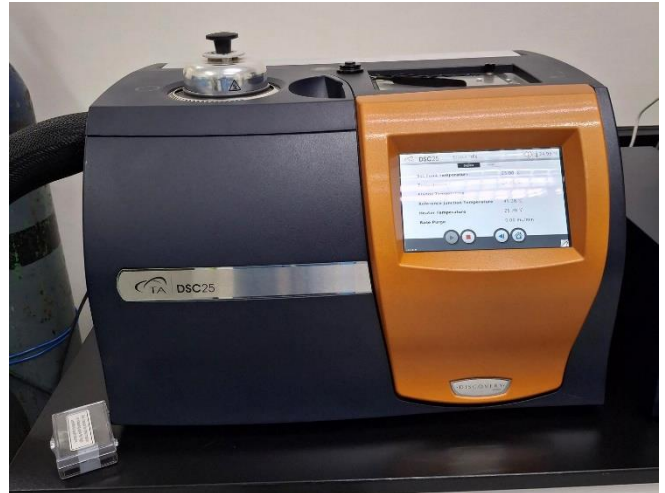
Fig. 5. Differential Scanning Calorimetry is used to determine the curing percentage of the adhesive.
