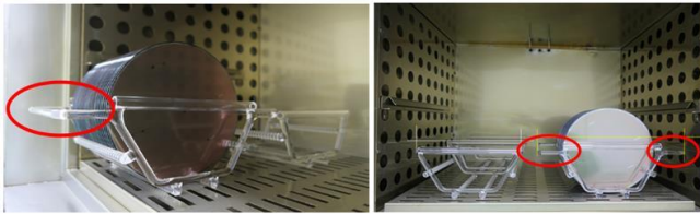
Figure 4. Redesigned quartz cassette (Revision 1)
