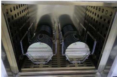
Figure 5. New quartz cassette design inside the oven chamber.
