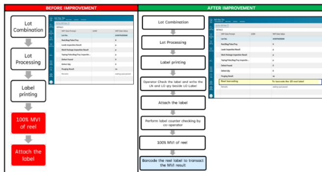
Fig. 6. To control the interchanging of process through Barcoding the reel label to transact the MVI result, an enhancement of MES by Barcoding the reel label to transact the MVI result is added as countermeasure.
