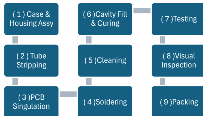
Fig.6 Connector Assembly Process Flow
