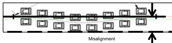
Fig. 1.6. Singulation with High fiducial deflection
