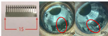
Fig. 4. From left to right: finger stock original length of 15 fingers; finger stock original length when rolled and assembled into mirror mount with overlap; finger stock reduced into 14 fingers, with no more overlap but with gap.
