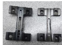
Figure 20a. Warped Back-guide (left) and I-guide (right)
