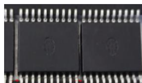
Figure 9a. Bent leads
