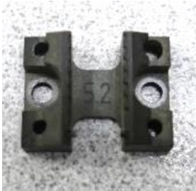
Figure 22a. Worn-out Contact Ledge
