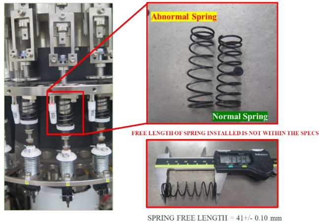
Figure 11. Force Testing Preparation Spring under observation will be elongated with actual measurement of 47.34mm and out of specs vs. Spring free length of 41 +/- 0.10mm.
