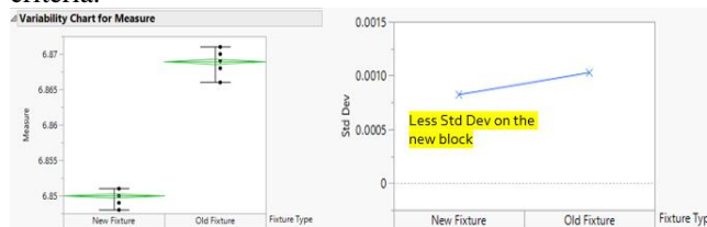
Fig.11 Less Standard deviation when changing the fixture block. GR&R results after implementing the change on fixture or block where the parts are placed when measured. The results showed improvement also but still failed based on criteria.
