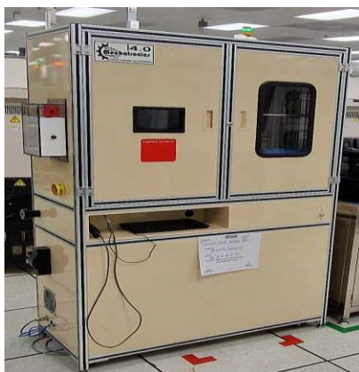
Fig. 11. AutoCap prototype developed based on TRIZ-derived design principles. This is the result of integrating TRIZ-based features for automated capillary handling.
