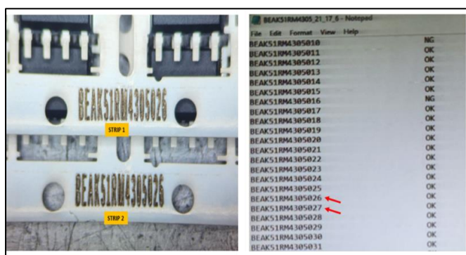
Fig. 5. Actual Strips Marking vs Mark History at Machine PC
