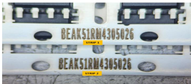
Fig. 1. Identical 2DID codes to different Lead Frames
