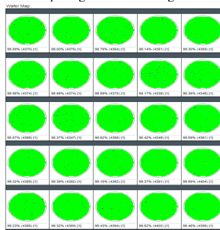
Fig.14. Production wafer maps with yield obtain after split site testing implementation
