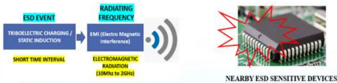
(Figure 3: Shows the ESD event are radiating frequency thru the air, this radiating frequency is the EMI that can damage an ESD sensitive devices.)
