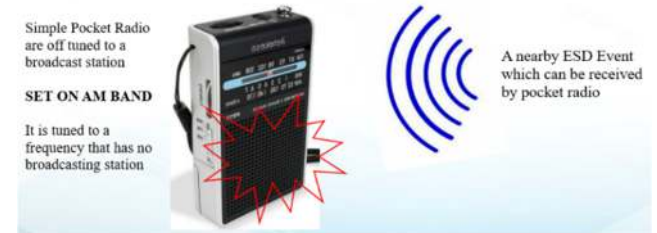
(Figure 5: A crackling or popping sound is heard on the background which an indication of interference near the area where the radio is placed.)
