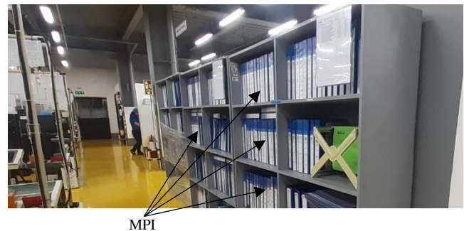
Fig. 3. Shelves of Paper-Based Work Instruction or Manufacturing Process Instructions (MPI). Filed in a binder and displayed in the production area.
