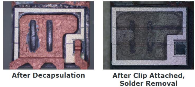
Figure 4. Decapsulation of the failed unit
