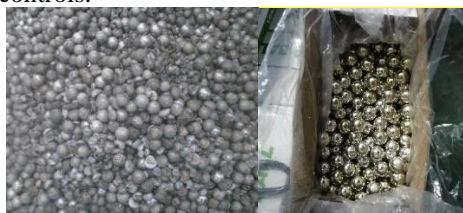
Fig9. Passivated Anode balls (Left); Fresh Anode balls (Right)
