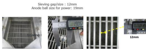
Figure 23: Tin Anode Sieve and its dimension
