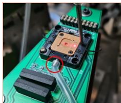
Fig. 21, Air Blow on Socket Pogo Pins
