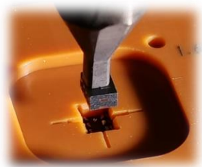
Fig. 10, Misaligned Turret Pickup Head vs. device A
