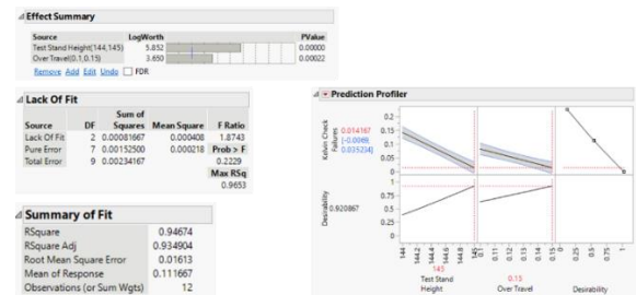
Fig. 24 Based on the profiler of the refined model with predictive capability of 94% the best parameter combination to be used to achieve maximum desirability are, Over Travel= 0.15 mm & Stand height = 145.
