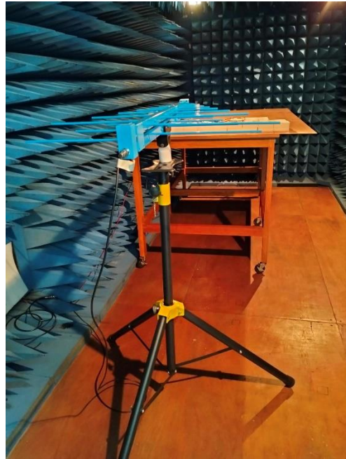
Fig. 6. Radiated emission using LPDA sensitivity range from 250 MHz to 1.3 GHz.
