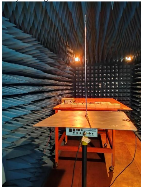
Fig. 4 Radiated emission setup. Monopole sensitivity range from 150 kHz to 30 MHz.
