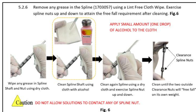
Figure 26. Defined process for proper cleaning of Spline.
