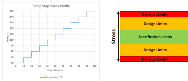
Fig 5. Temperature Step Stress Test Profile
