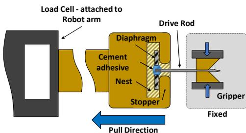
Figure 10. Test Fixture Design and Mechanism.
