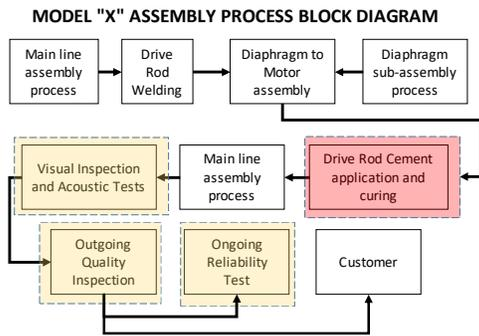
Figure 4. Model “X” Assembly Process Block Diagram.
