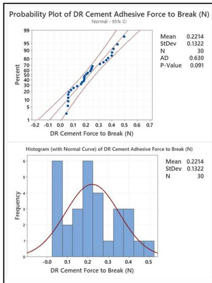
Figure 12. Drive Rod Cement Adhesive Pull-out Data – F, Force to Break in Newtons.
