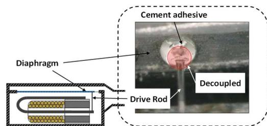
Figure 3. Actual image of the representative BA that failed the ORTs.
