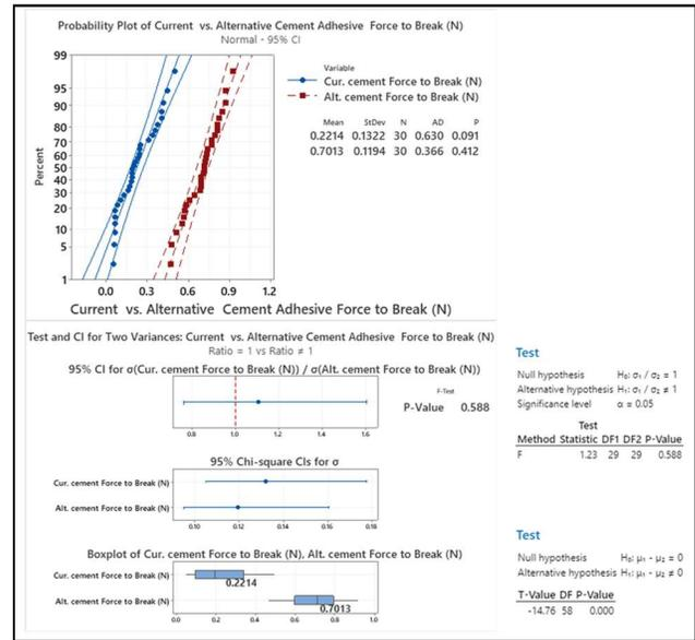
Figure 13. Current Cement Adhesive vs. Alternative Cement Adhesive Force to Break (N) comparison.
