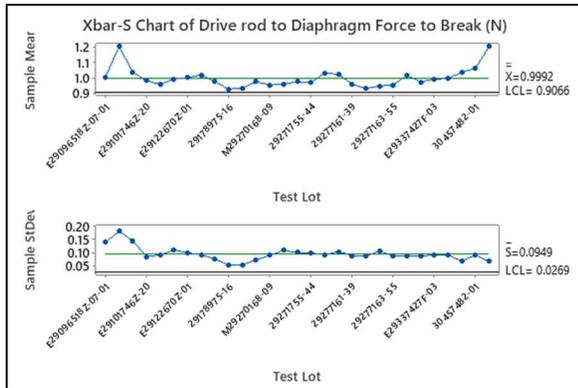
Figure 15. Xbar-S Chart of the drive rod to diaphragm pull-out test data
