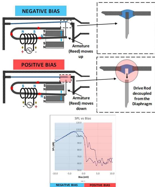
Figure 2. Sound Pressure Level vs. Voltage Bias of a Balanced Armature Driver with a mechanically de-coupled Drive Rod to Diaphragm connection.
