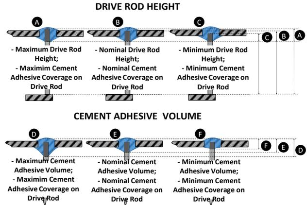
Figure 6. Drive rod cement adhesive coverage variability.
