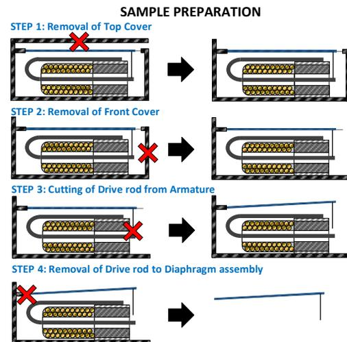
Figure 8. Sample preparation and disassembly process.
