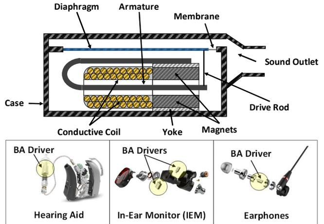
Figure 1. Cross-section of a Balanced Armature Driver and its typical designated usage.
