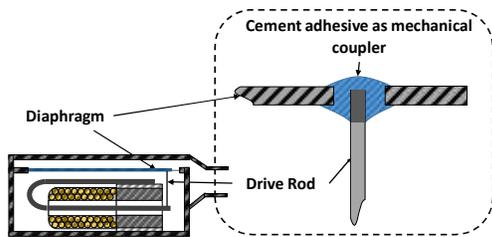
Figure 5. Extreme close-up view of the drive rod to diaphragm connection.
