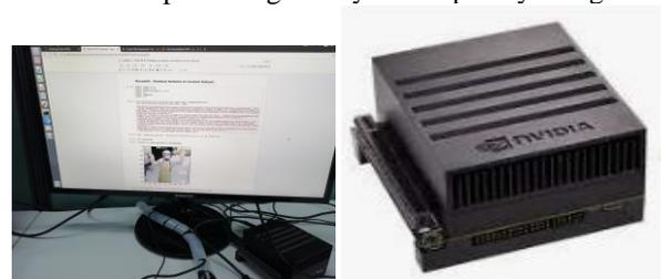
Figure 8. Hardware Set-Up for Machine Learning. The photos show the NVIDIA Jetson Tegra Xavier that was used in the data extensive processing.
