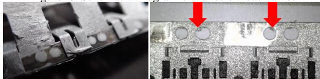
Figure17. Actual image of belt simulated with flakes.
