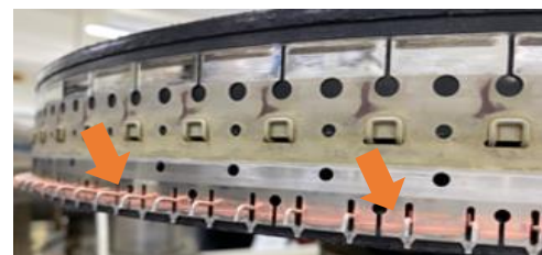
Figure9. Discolored belt due to Galvanic Corrosion
