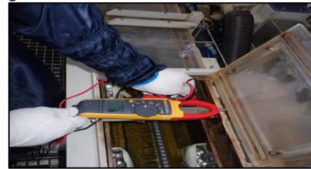
Figure 12. Measurement of rectifier output
