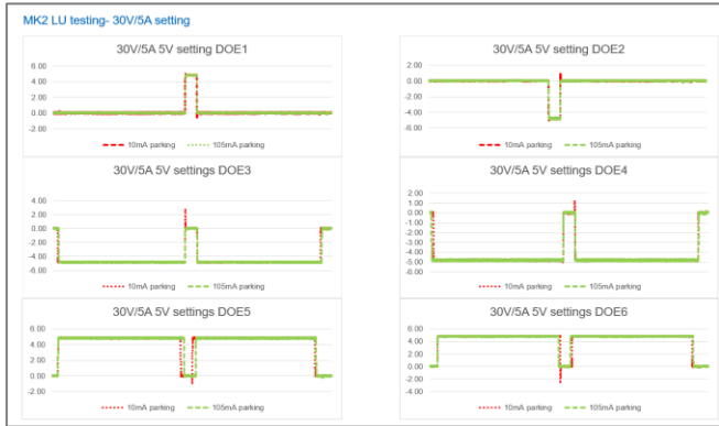
Fig. 2. 30V/5A waveform measurement for 10mA and 105mA parking.
