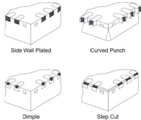
Fig. 1. Solderable sidewall options for wettable flank QFN<sup>8</sup>
