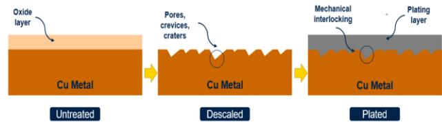
Fig. 6. Descaling process
