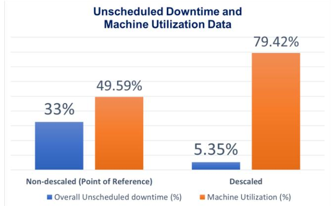
Fig. 11. Non-descaled vs descaled unscheduled downtime and machine utilization data
