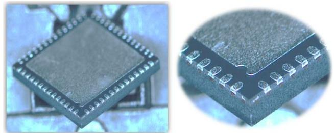
Fig. 2. wettable flank QFN with step cut
