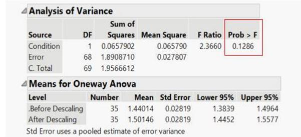
Fig. 14. One way analysis of stand-off by leadframe condition
