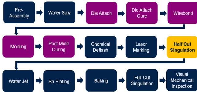
Fig. 3. Assembly process flow for wettable flank QFN packages
