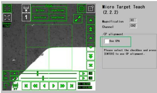
Fig. 5. Contrast pattern alignment in singulation
