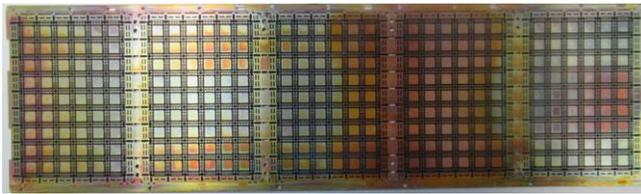
Fig. 4. Leadframe with surface oxidation
