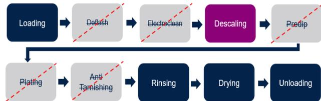
Fig. 7. Process flow inside Sn plating machine, descaling activated
