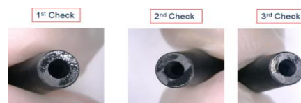
Figure. 20. Turret Tip Checkout after cleaning
