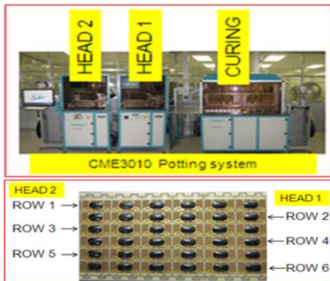
Fig. 4. Head 1 encapsulates the even rows while Head 2 encapsulates the odd rows.
