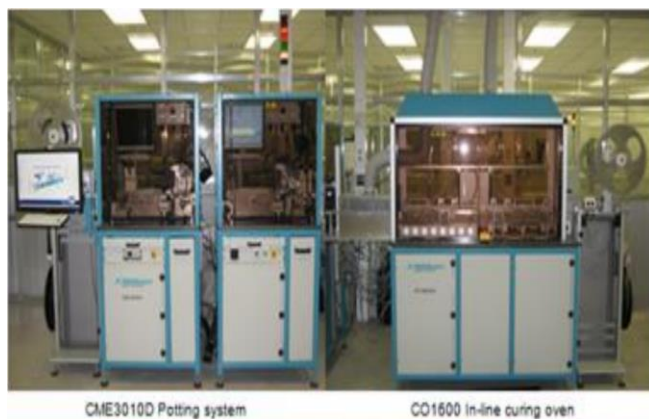
Fig. 1. CME3010D Potting System and Inline Curing Oven
