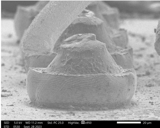
Fig. 1. SEM image on the wire break on neck observed after TC1000.
