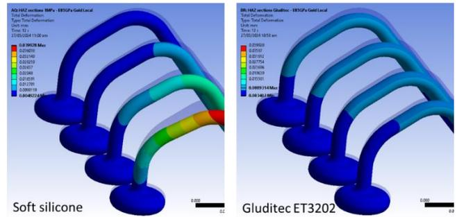
Figure 5. Deformation plot comparison on soft silicone and hard epoxy
