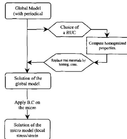
Figure 2. Process flow chart for multi-level and homogenization technique.
