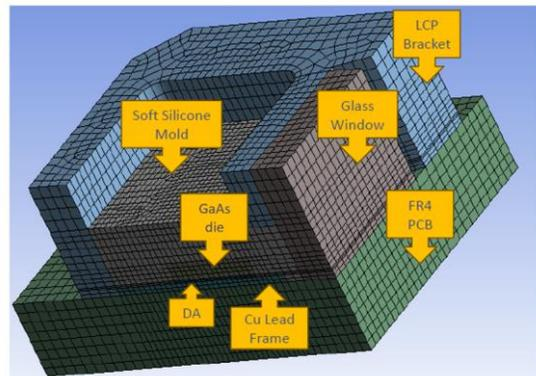
Figure 3. 3D drawing of area of interest showing the different material interface
