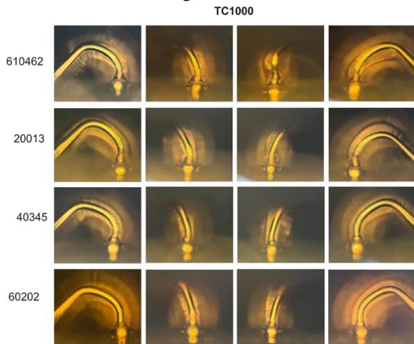
Figure 7. TC1000 visual inspection on units with soft silicone encapsulant (Note: Unit 90303 was subjected to decapsulation at TC800).
