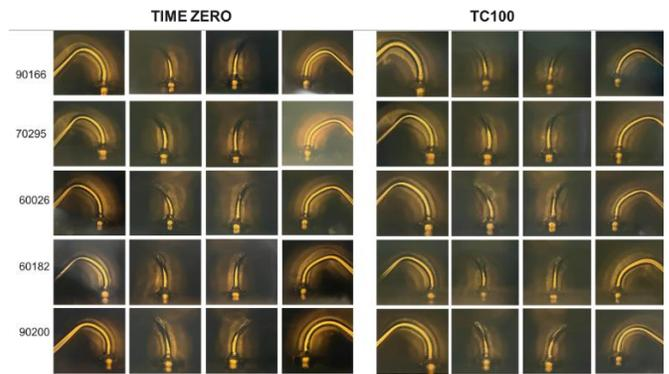
Figure 8. Time zero and TC100 comparison on automotive units processed with hard epoxy encapsulant
