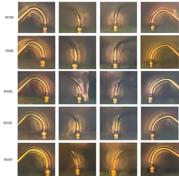
Figure 9. TC800 visual inspection on automotive units with hard epoxy encapsulant
