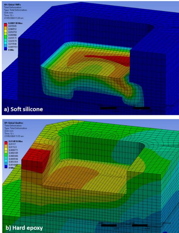
Figure 4. Global deformation plots of a) soft silicone and b) hard epoxy
