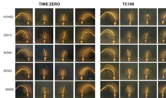
Figure 6. Time zero and TC100 comparison on automotive units processed with soft silicone encapsulant
