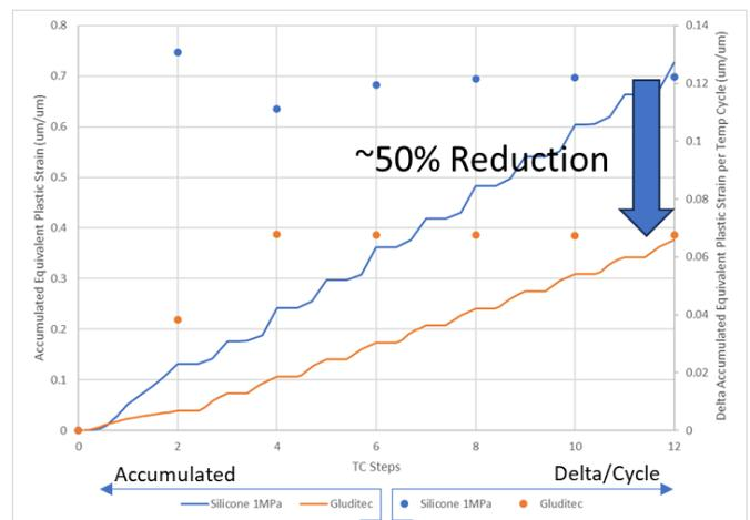
Figure 6. Accumulated plastic strain and delta per cycle of soft silicone and hard epoxy
