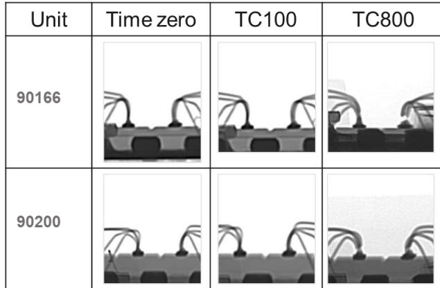
Figure 10. X-ray inspection of hard epoxy at time zero, 100 cycles, and 800 cycles
