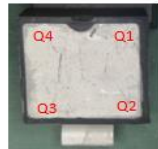
Fig 9: Heavy mold flashing on lead side of the molded strips
