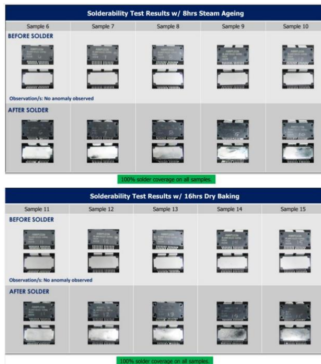
Fig.6. Sample photo of OMP1 undergone solderability test
