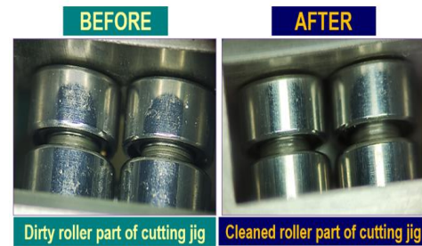
Figure 11. Dirty vs. Cleaned roller part of Cutting Jig
