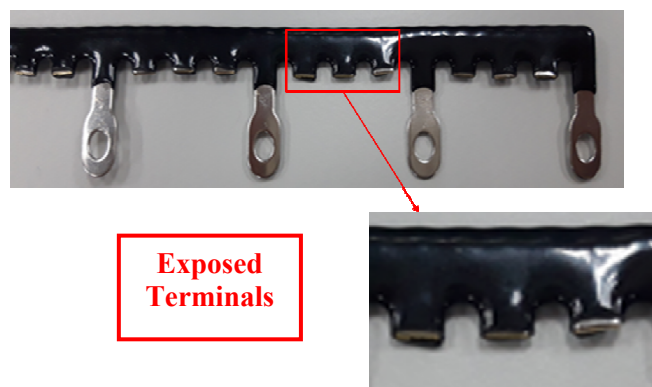
Figure 3: Exposed terminals due to no good cutting of shorting bar.
