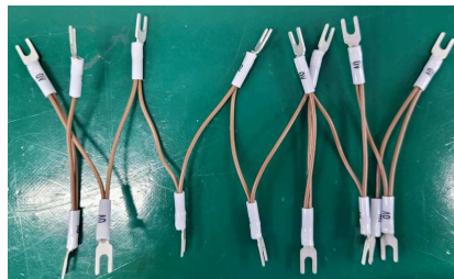
Figure 6b: Sample wire jumpers for DC power supply (0V)
