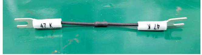
Figure 7: 47k \Omega resistor with insulation
