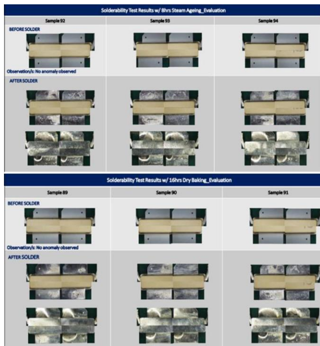
Fig 4.8 Solderability tests results for 0Hr dip and look, post dry-bake and post steam-age.
