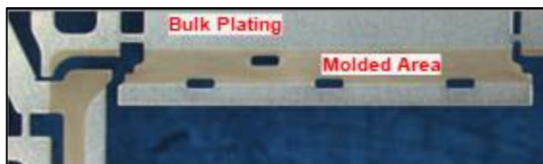
Fig 4.2 The two primary surface finishes of the leadframe, the bulk plated area and the mold plated area
