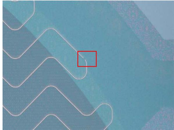
Figure 2: 1000x magnification Broken trace length
