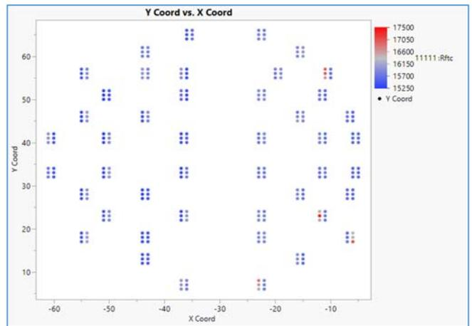
Figure 12: Bin Failure topography on Wafer Map (DCR Sampling for Product A)
