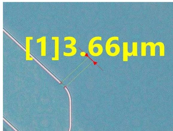
Figure 3: 1500x magnification of Broken trace length
