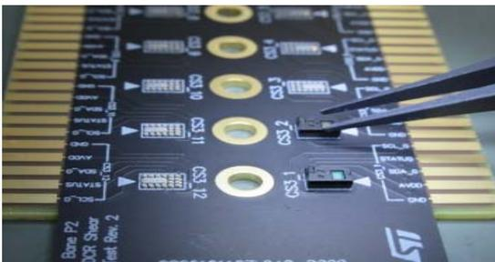
Figure 6: Manual Placement of unit
