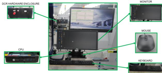
Figure 5: Interface of PC in performing Manual DCR Testing.
