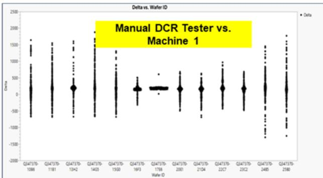
Figure 10: Correlation on Manual DCR Tester and Machine 1
