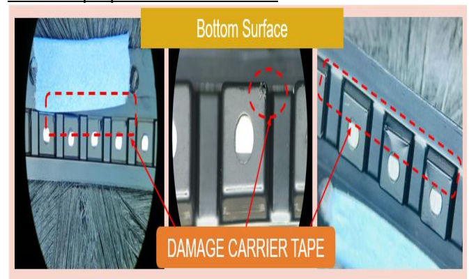
Figure 2. This defect can be seen that bottom corner pocket of DFN8 2X2 that has pointed corner pocket compare to other package type that has curved/rounded bottom corner pocket
