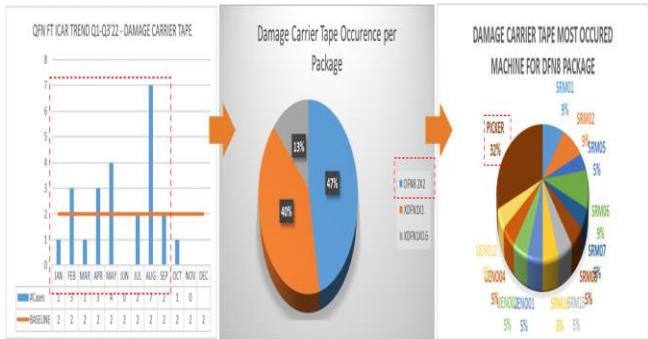
Figure 4. Damage Carrier tape cases, DFN8 2X2 and Picker Machine is the top.
