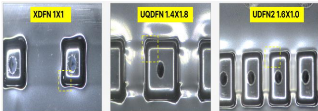
Figure 6. Design with curved/rounded Above the 3 samples of Carrier Tape were the bottom corner of the pocket has curved/rounded corner
