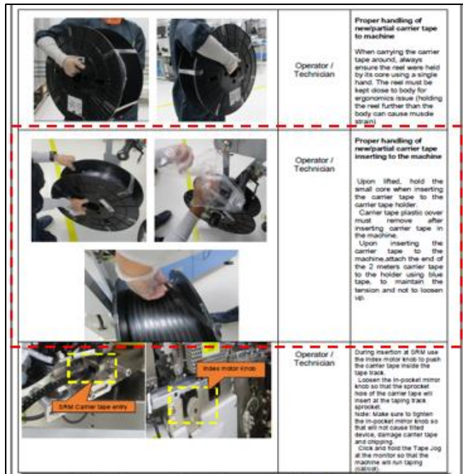
Figure 8. No detailed procedure on proper installation of carrier tape at the handler and can contribute to damage carrier tape
