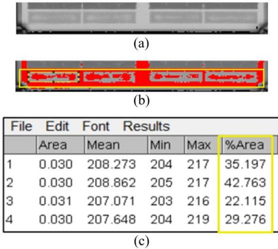
Fig 1. (a) SCAT images of capacitor dies, (b) processed SCAT images on ImageJ showing detected delaminated area and (c) calculated percent delaminated area per die.
