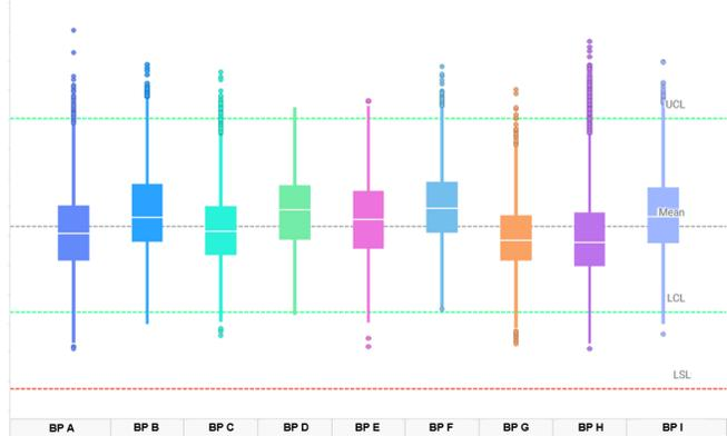
Fig. 4. Box plot of ball shear response per bond program for Chart PC-AI
