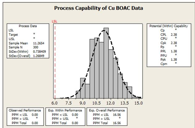
Fig. 10. Process capability analysis on shear per area (SPA) data for Cu/BOAC devices.
