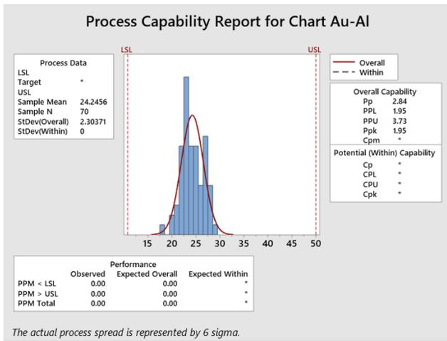
Fig. 9. Process capability analysis on lead lots processed with bond parameter X = 220.
