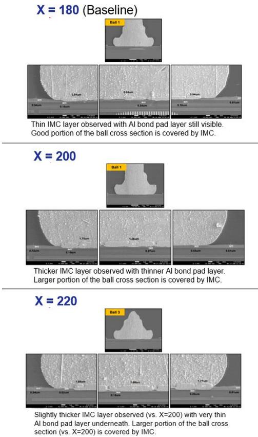
Fig. 8. Cross section analysis on units processed at bond parameter X = 180 (baseline), X = 200, and X = 220, highlighting the Al bond pad thickness.
