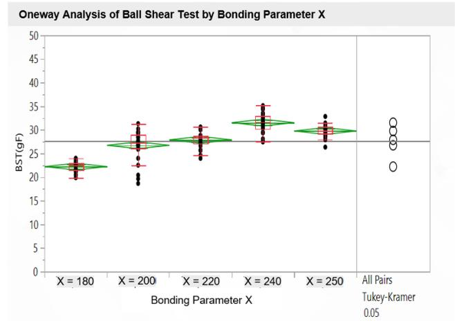
Fig. 6. One-way ANOVA of ball shear readings with increasing bond parameter X.
