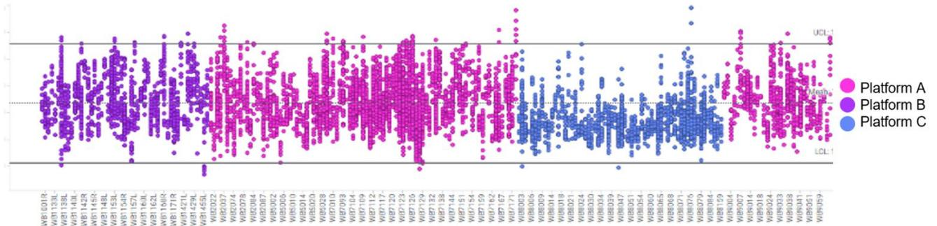
Appendix B. Scatter plot of ball shear readings per tool and categorized according to the tool platform used.
