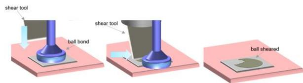
Fig. 1. Illustration of the ball shear process. Shear tool applies lateral load on the ball bond and gives a reading/measurement in gram-force (gF).
