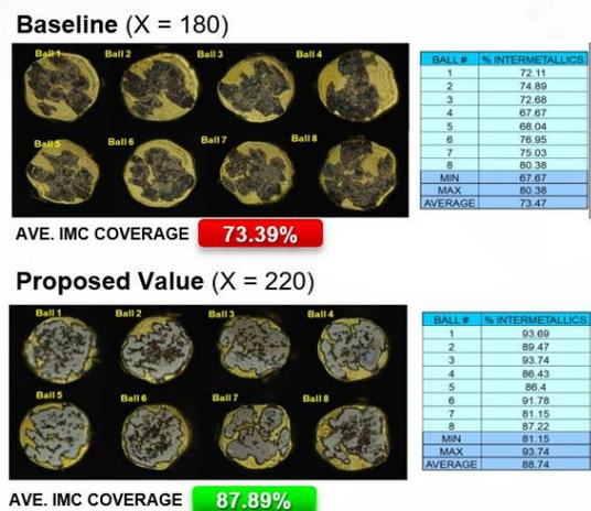
Fig. 7. Intermetallic coverage on units processed at baseline parameters (X = 180) versus units processed with increased bond parameter X (X = 220).
