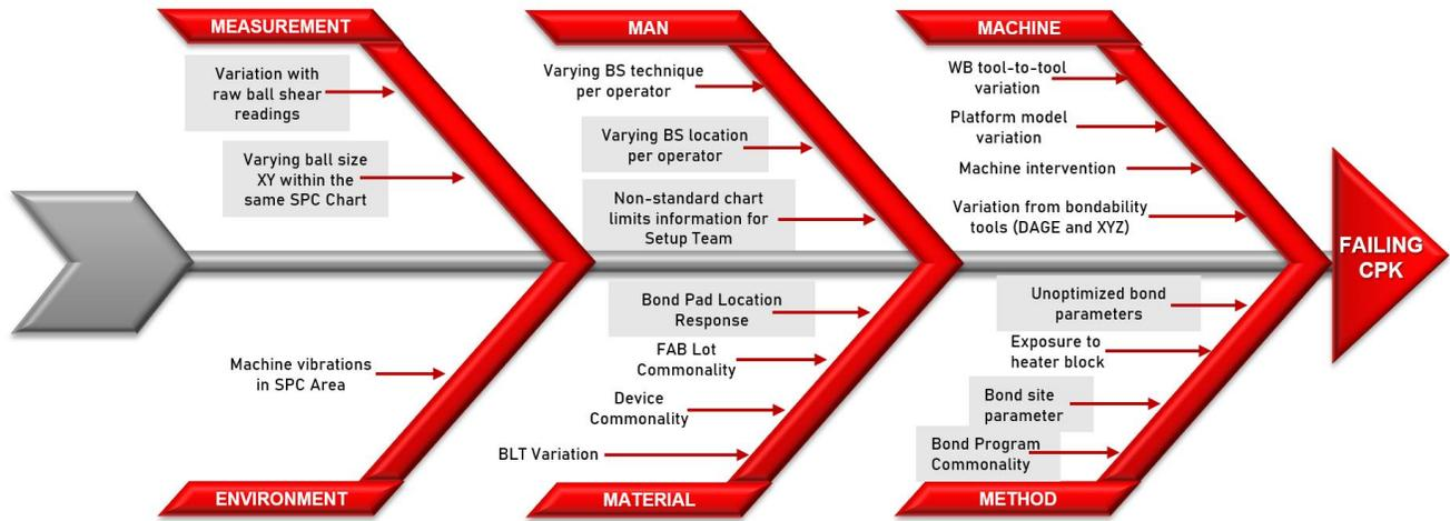
Appendix A. Fishbone diagram of all possible man-, machine-, material-, method-, measurement-, and environment-related factors contributing to failing CpK of ball shear charts.
