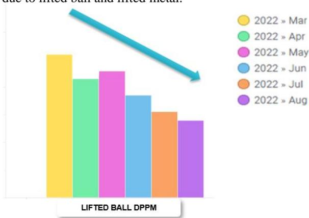
Fig. 11. Lifted ball defective parts per million trend upon implementation of defined actions.
