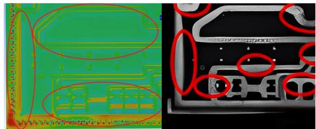
Figure 8: Simulation Stress Result and TST 50 Cycles comparison.
