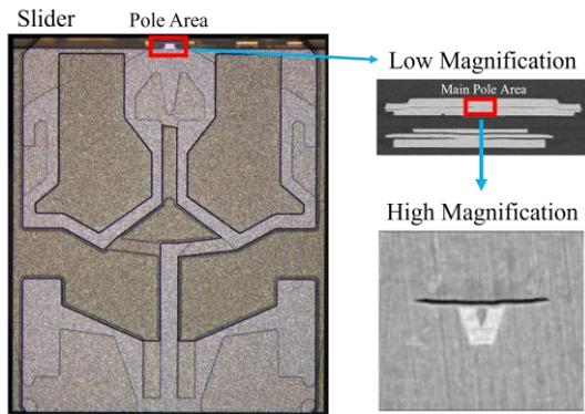
Fig. 4. Sample CDSEM images for low and high magnification inspection process.
