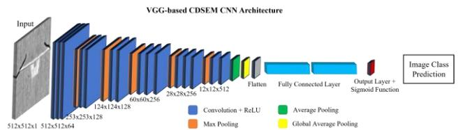
Fig. 5. VGG-based CDSEM CNN architecture.
