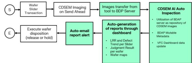
Fig. 2. The updated project flow with automation on CDSEM inspection and report generation through dashboards and email reports.
