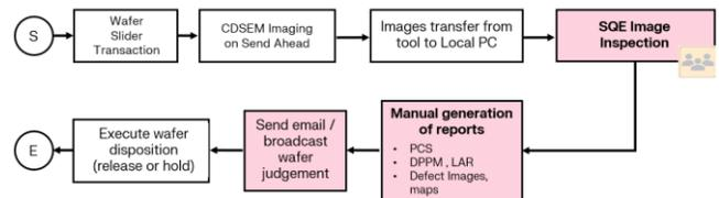
Fig. 1. Traditional CDSEM Manual Inspection Flow. Manually generated reports contain the following: Process Control Sheet (PCS), Defects Parts Per Million (DPPM), Lot Acceptance Rate (LAR), Defect Images, and Wafer Map.
