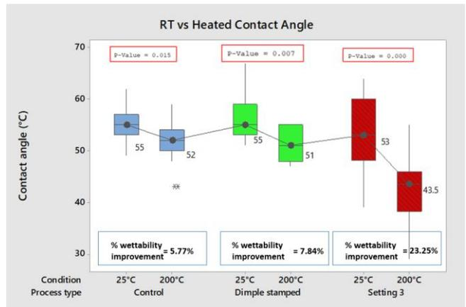
Figure 6: Boxplot contact angle at 25°C and 200°C
