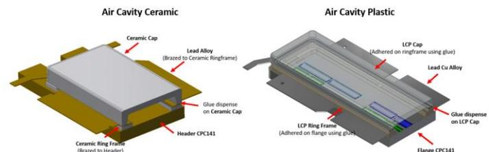
Figure 1. Air cavity packages
