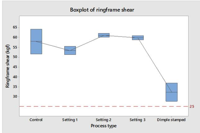
Figure 8: Zero-hour ringframe shear
