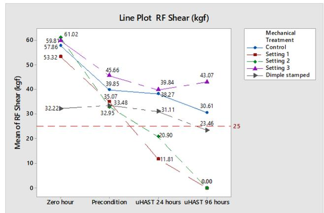
Figure 10: Zero-hour to uHAST Ringframe shear readings
