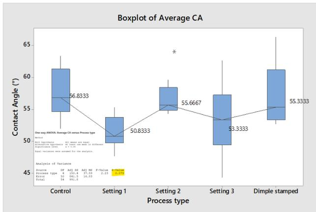
Figure 5: Boxplot contact angle at room temp
